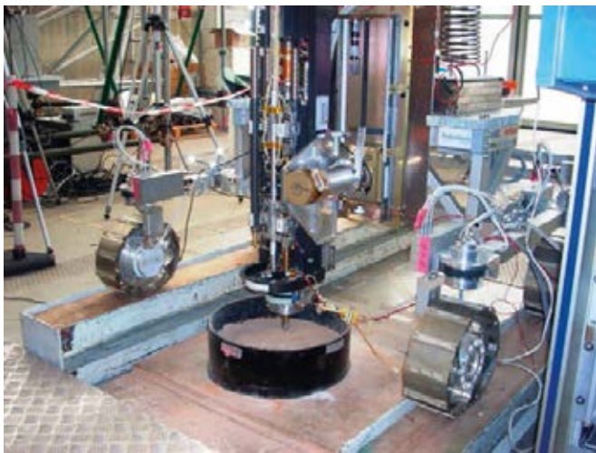
The Drill System integrated on to the Exomars Rover breadboard during the relevant test campaign.
