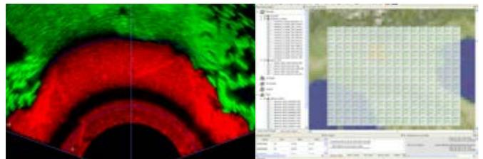
MARS can switch at runtime for training purposes from the radar image (left image), to Surface Material Codes used for reflectivity computations (centre image), to altimetry information (right image) used for occultation calculations.
