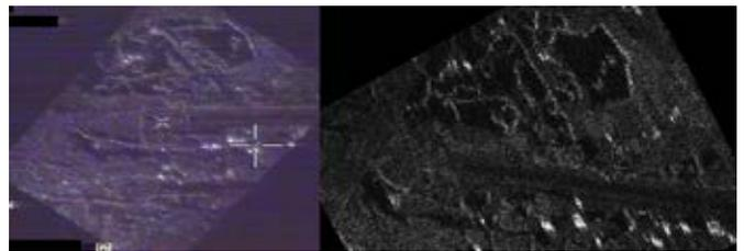
Comparison between a true Squinted Spotlight Doppler Beam Sharpening (SpDBS) image (left) and the corresponding real-time MARS simulation (right) using FFT processing (18 meters resolution on the Manching airport).
