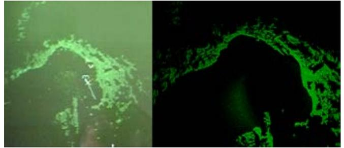
Comparison between a true Real Beam Ground Mapping (RBGM) radar image (left) and the corresponding real-time MARS simulation (right) using a non-coherent processing (Tyrrhenian sea and Coarse island).
