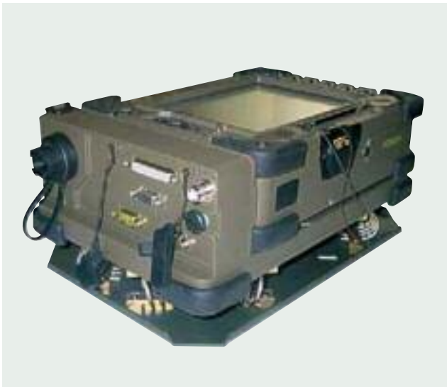
LRT-330 INSTALLED ON BA-330 SHOCK ABSORBING BASE
