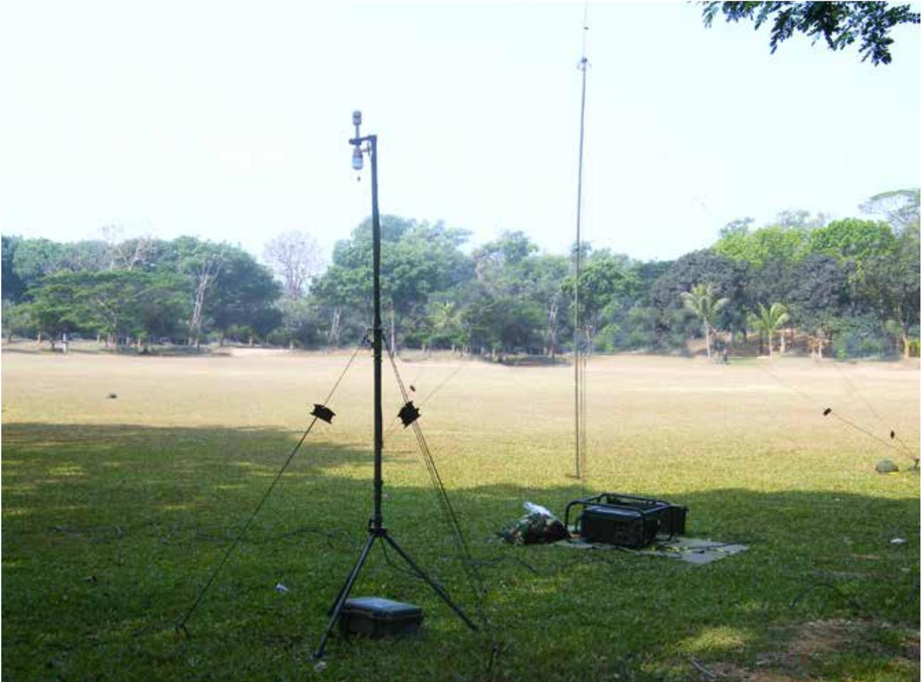
HALO is an extremely versatile system. It can be deployed in any configuration and in areas where there is limited space. SPs do not need to be laid out according to any particular template. GPS provides sufficient accuracy for HALO survey. A computer-based deployment aid assists the user in optimising area coverage and communications. This flexibility enables HALO to be used successfully in cities and other complex terrains.
