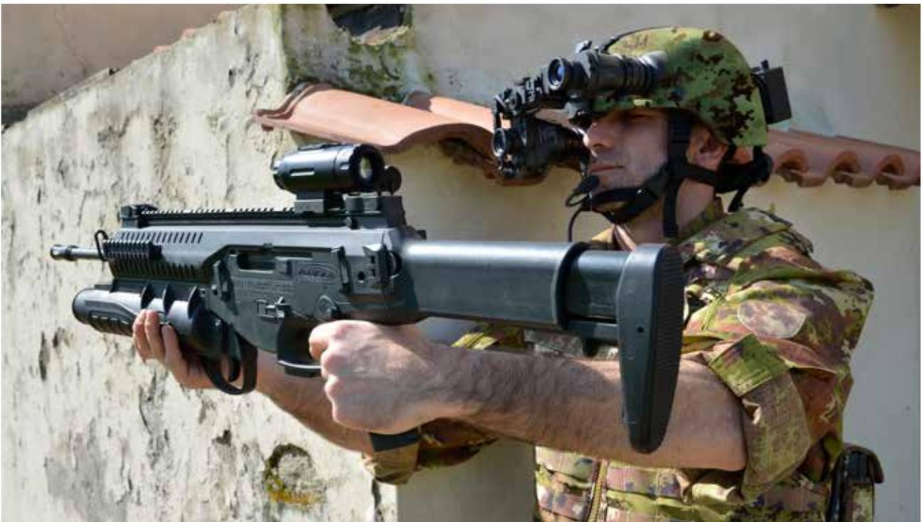
MINISIGHT combines day and night video channels and, as ASPIS, can be connected to the soldier's computer via a Bluetooth link. In conjunction with NIMOS enables soldiers to observe and fire around the corner.
