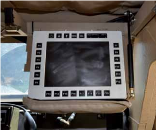
Typical 10.4" MDU installation for vehicle commander
