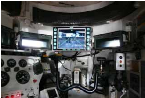
8.4" DDU fitted at vehicle driver's position
