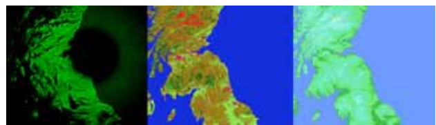
MARS can switch at runtime for training purposes from the radar image (left image), to Surface Material Codes used for reflectivity computations (center image), to altimetry information (right image) used for occultation calculations.
