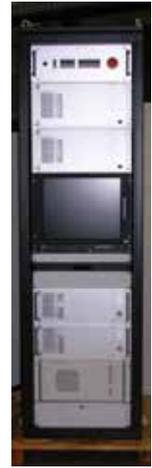
The Transceiver and Processor Unit can be installed either in a single indoor Rack Unit close to the Antenna Unit, or split in two Rack Units. One is installed outdoors, near the Antenna Unit, and the other indoors, even at large distance from the other. This second option can be useful in case of very high tower by maintaining the simpler, low power and less expensive SMR installation arrangements.
